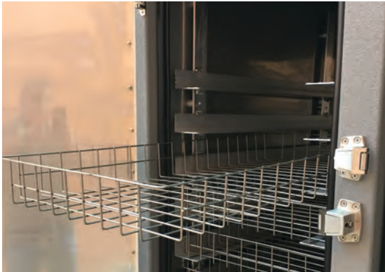
Slide-out racks on the hot side of the meal storage box.
