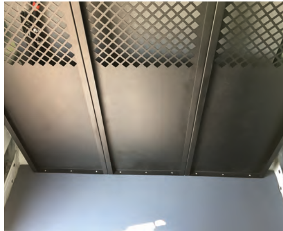
Durable, steel partition in front of the food box section. This package allows for a storage area behind the 2nd row passenger seats.
