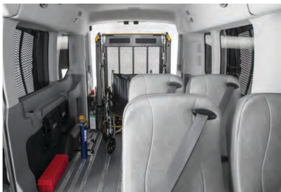
Inside view of paratransit van with SmartFloor system and wheelchair lift in rear location.
